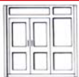
GDD or FDD Double timber doors with transom lights and side infill panel. Width (double module) - 8'(2400mm). Door height 6'8" (2040mm). Door width 4'10" (1476mm). Glazed or flush.
