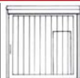
S8 Timber sliding door available in sides of 8'3"(2.5m) and 10'0" (3.0m) eaves height buildings only. Width 7'6"(2276mm). Height 7'5"(2270mm) for 8'3"(2.5m) eaves height and 9'1"(2770mm) for 10'0"(3.0m) eaves height.
