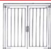
F8 Timber hinged double doors for side or gable (side door not available on 6'8" (2.20m) eaves height buildings). Width (double module) - 8' (2400mm). Opening width 7'2" (2194mm). Height of side doors is 7'5" (2260mm) for 8'3" (2.5m) eaves height and 9'1" (2770mm) for 10'(3m) eaves height. Gable door heights for the 3 eaves heights are 6'2"(1880mm), 8'1"(2470mm) and 9'9"(2975mm) respectively.
